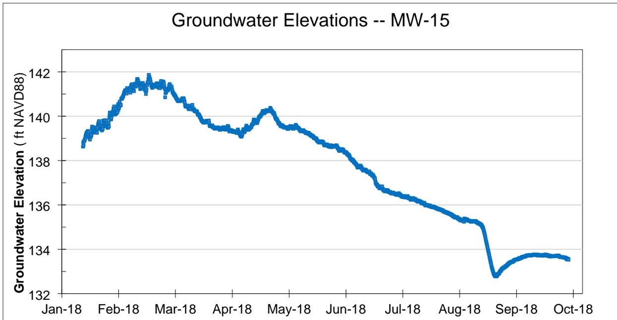
Figure 9f. Groundwater Elevations in Lacey S-16 (Qva)
