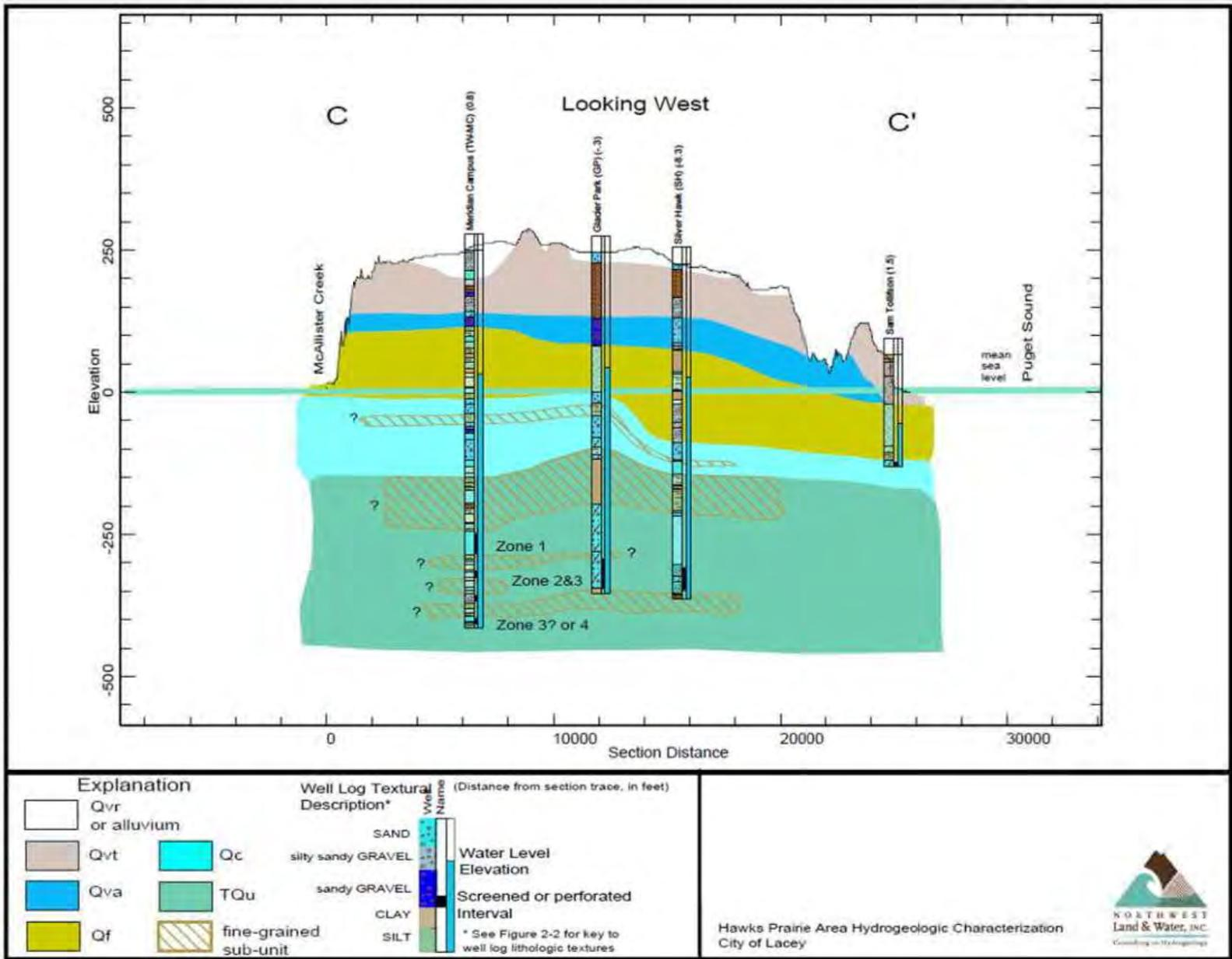
Hydrogeologic Cross Sections, NWLW 2008
