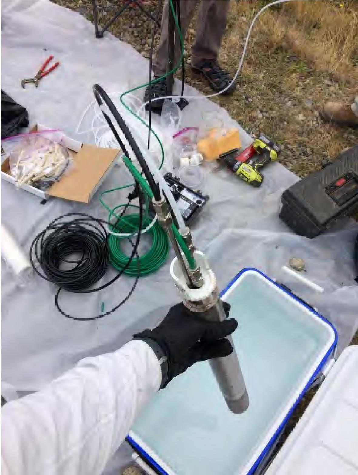
**Figure 3-3. Photograph of Lysimeter Prior to Installation.**
