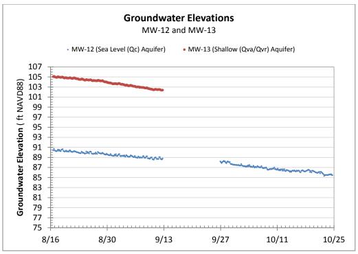
Figure 4-10. Groundwater Elevations MW-12 and MW-13
