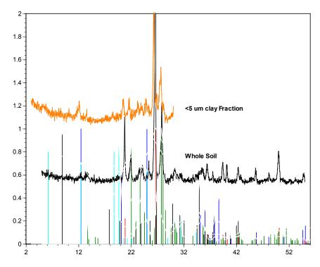
Figure 2: XRD patterns for **West Lysimeter** sample w/ stick patterns for **quartz (red)**, **feldspars** (green), **kaolinite (blue)**, **mica (black) and chlorite (Cyan**)
