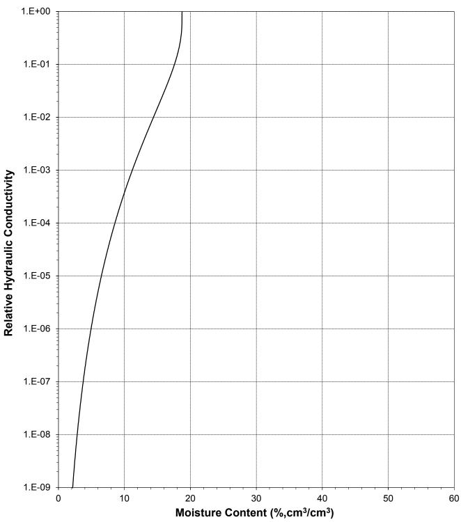
Plot of Relative Hydraulic Conductivity vs Moisture Content
