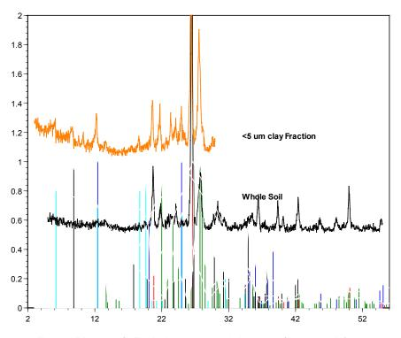
Figure 1: XRD patterns for East Lysimeter sample w/ stick patterns for quartz (red), feldspars (green), kaolinite (blue), mica (black) and chlorite (Cyan)
