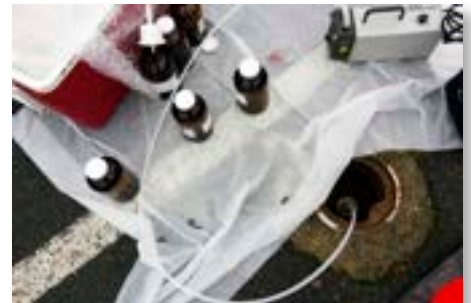
The tracer test tracked movement of reclaimed water
