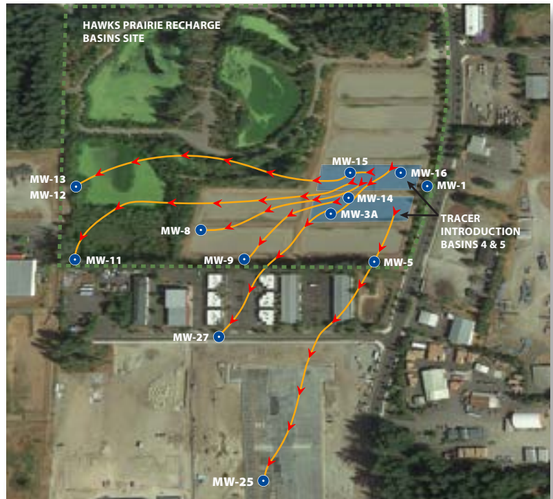
Tracer test data confirmed where infiltrated reclaimed water traveled after mixing with groundwater
