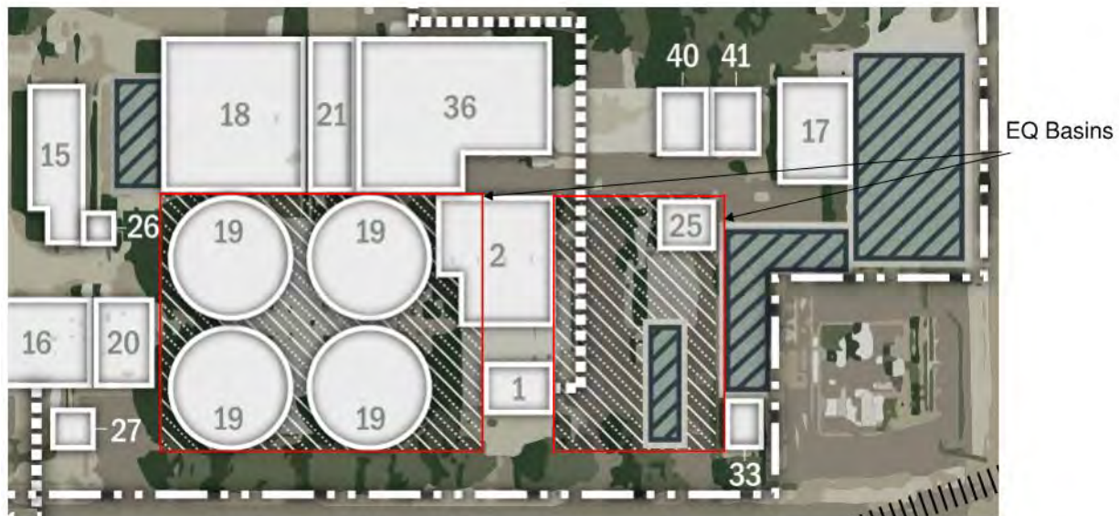
Figure 3-2. EQ basins (hatched)
